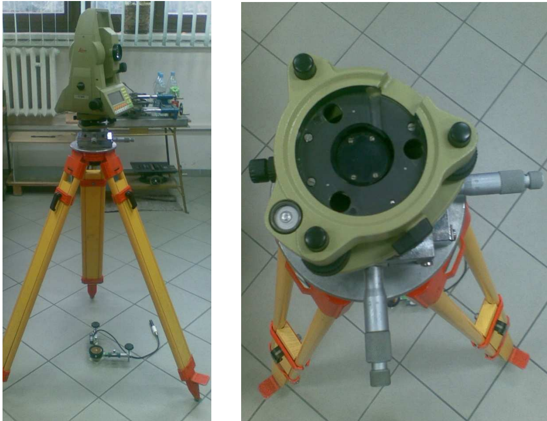
Fig. 5 Electronic tachymeter TC1800 centering over reflective optical fiber adapter
