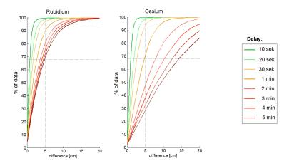
After 10 sec. 95% of corrections degrades < 2 cm, 30 sec. < 5cm Correction for satellites with Cesium clocks degrades significantly faster.
