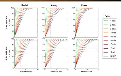
After 1 min. 95% of corrections degrades < 2 cm; 4min. < 5cm Correction for satellites with Cesium clocks degrades slightly faster.
