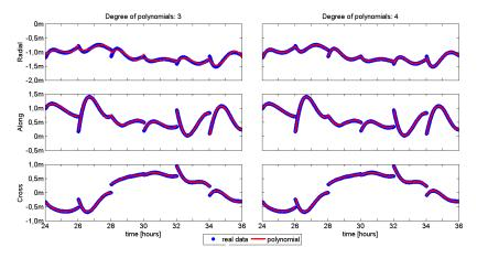
Polynomials of degree 3 and 4 fited into 2-hour time series of orbit correction data (PRN 1: IIF,Rb)
