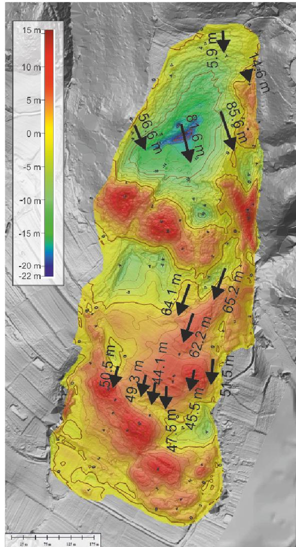
Fig. 2. Landslide deformation model calculated on the basis of photogrammetric data from 2009 year and airborne laser scanning data of July 2010; horizontal displacements based on a comparison of aerial photographs
