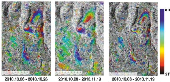
Fig. 5. Sample interferograms from satellite data acquired by TerraSAR-X
