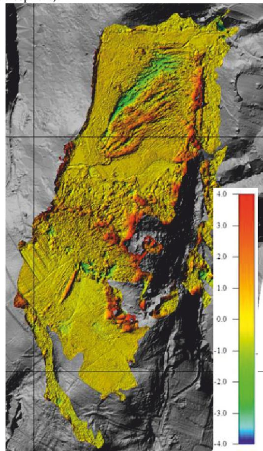
Fig. 4. The dynamics of landslides between July 2010 (measured with ALS) and May 2011 (measured with TLS).
