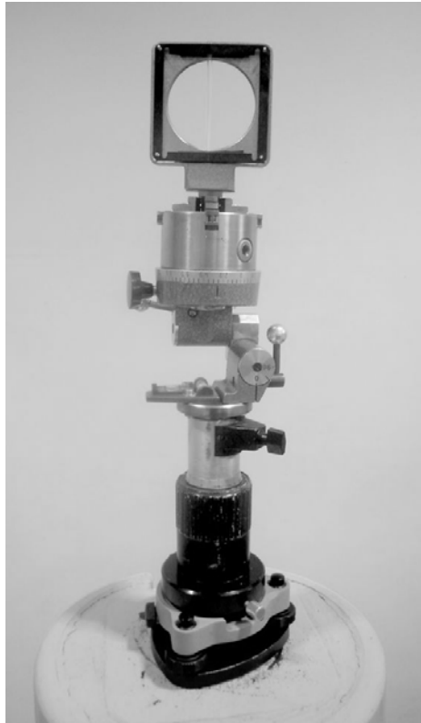
Fig. 2. A prototype of a universal simulation table on a measurement post.
