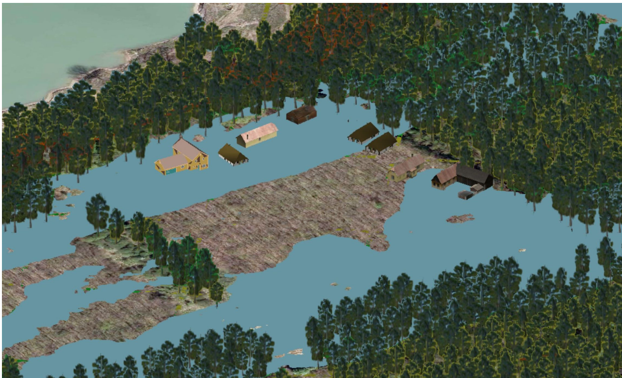
Fig. 4 Example of flood 3D visualization for the area with buildings and vegetation
