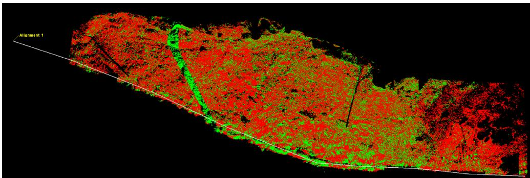
**Fig. 6** Point clouds from two epochs (green – first measure, red – control measure) and line of cross section
