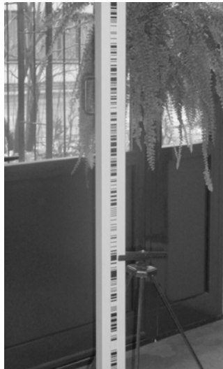
Photo 7. Code rod set on a test bench mark
