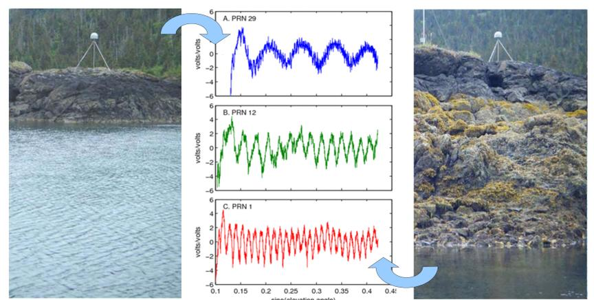
Figure 2 (above): photograph of PBAY GNSS site at low and high tides (left and right panels, respectively); SNR data (middle panel) for three satellite tracks at low, medium, and high tides.
