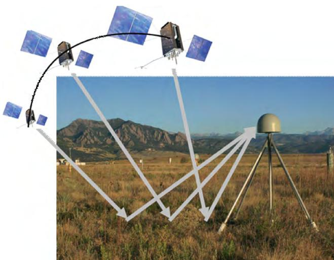
Figure 1 (left): as GNSS satellites rise and set in the sky, their reflections off natural surfaces (such as soil, sea, and snow) allow monitoring soil moisture, sea level, and snow depth, among other environmental targets.
