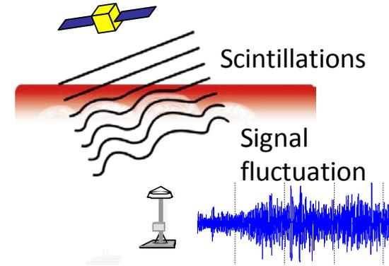
GNSS Signal is disturbed by ionospheric irregularities (plasma bubble) and may be lost in severe case.
