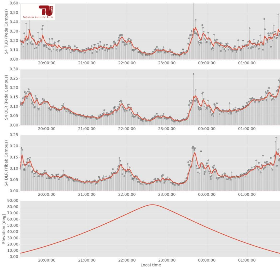
Signature (red line, exponentially-weighted moving average, window size: 3 min) of S4 indices (grey dots) calculated for satellite G24 from different scintillation processors in comparison to the averaged elevation.
