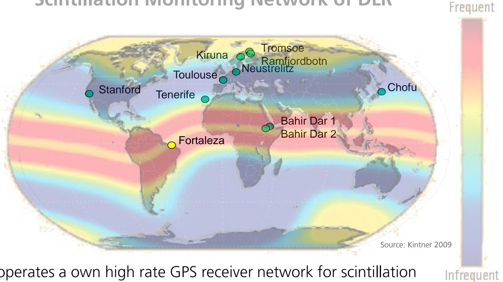
DLR operates a own high rate GPS receiver network for scintillation measurement from high latitudes (Kiruna /Sweden) down to equatorial regions (Bahir Dar/Ethiopia). Scintillation data of several stations provided in real time via IMPC/SWACI <http://swaciweb.dlr.de>
