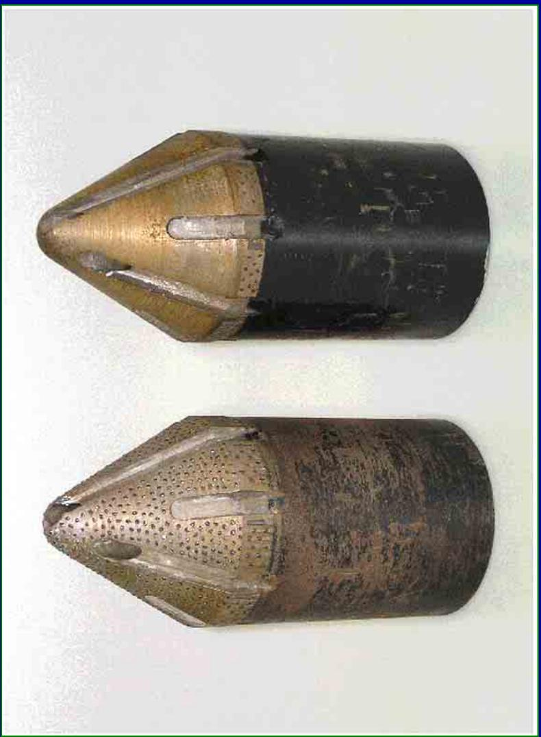
Special conical bit for preparing of borehole bottom
