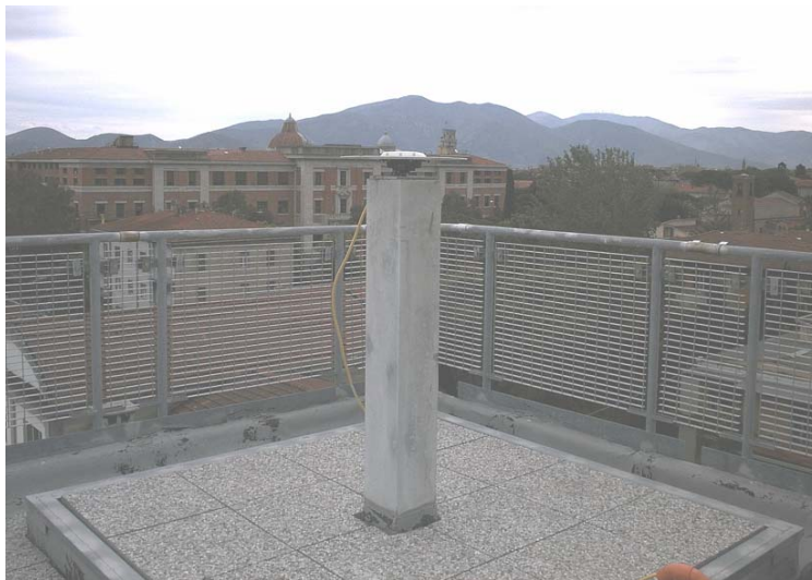
Fig. 1 – Materialisation of GPS permanent station of Pisa.
